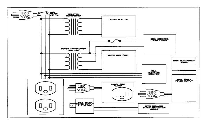
The power wiring for American Laser Games consists of both line voltage (120 VAC) and low voltage (<30) sections. The low voltage sections are split up into two areas, low voltage AC for the audio amplifier board and coin door lights, and low voltage DC for the main electronics board and optoisolator board. The line voltage powers the laser disk player, the main board power supply, the opto isolator power supply, the bill accepter and the video monitor through an isolation transformer.
