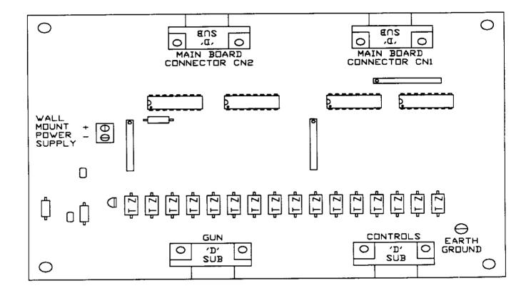
The Optoisolater board should be mounted within one and a half feet of the main electronics board. The four spacers are used to mount the board. Here are the steps to connect the optoisolator board to the American Laser Game system.
