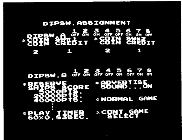
Self-Test - Dip Switch Assignment
