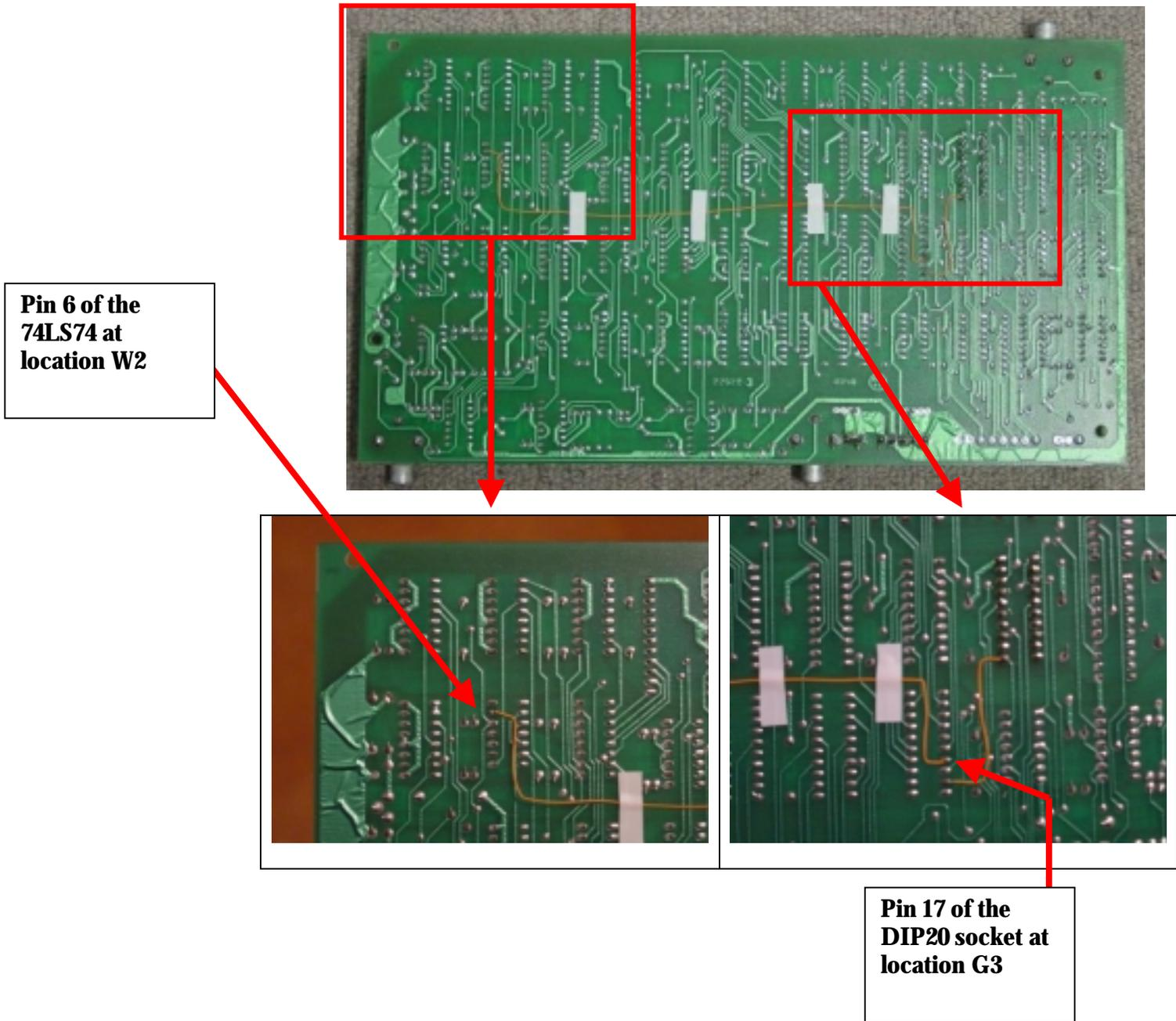
Be careful to look at the identifying text and labels on the top of the board, to be sure that you solder to the correct IC and pins on the underside.
