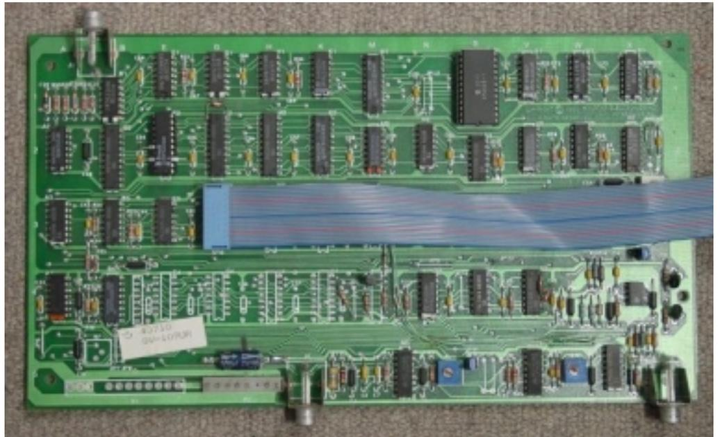
3. Solder the jumper wire from Pin1 of the 74LS244 at location E2, to pin 19 on the DIP20 socket at location G3
